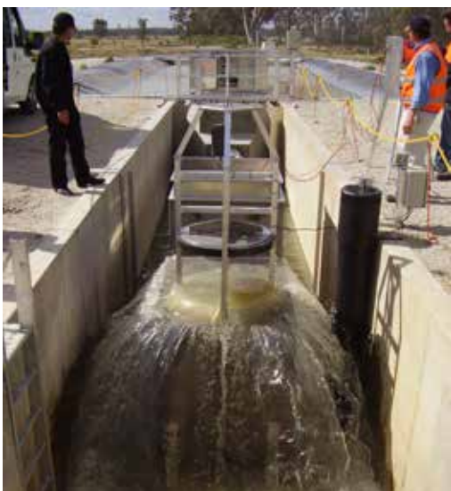
A new irrigation metering system being tested. Together with the water industry, NMI has developed a new irrigation meter standard to help manufacturers and users ensure consumption of irrigation water is measured accurately. (Photo: AWMA Pty Ltd)
